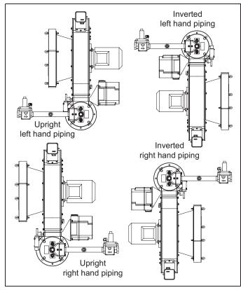
Figure 3.1. Configuration Selection and Motor Orientation Choice
