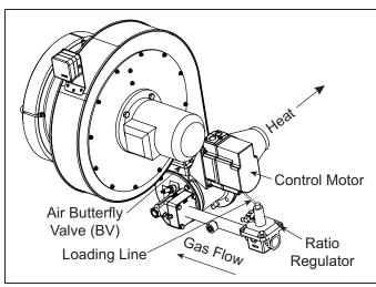
Figure 3.4. Basic Burner Components
