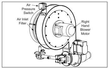
Figure 3.2. Burner Configuration & Motor Orientation Choice
