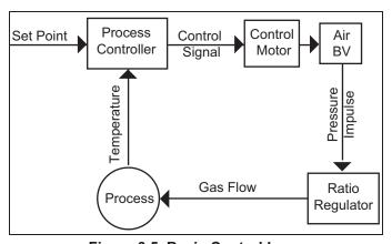
Figure 3.5. Basic Control Loop
