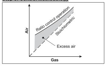
Figure 3.3. Air: Gas Flow
